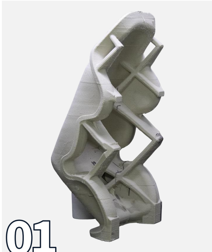
3D Printed Shell with Mold Inside
