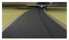
Close-up of Roboze's UFO-extruder depositing a porosity-free composite layer. An automated casting system dispenses the A&B components according to the required ratio
