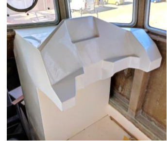
3D printed ergonomic dashboard produced without a mold. Printed in 8 hours only ! With traditional production, it would take over 2 weeks just to create one mold
