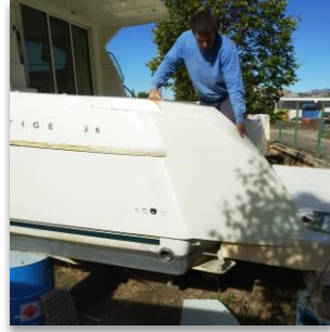
3D printed symmetrical stern extension by Velum Nautica. using integrated slicer software
