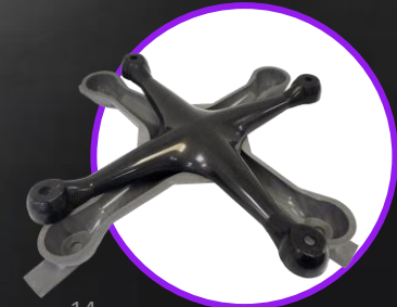
14 A mold for drone manufacturing produced using a Massivit printer and Sika materials
