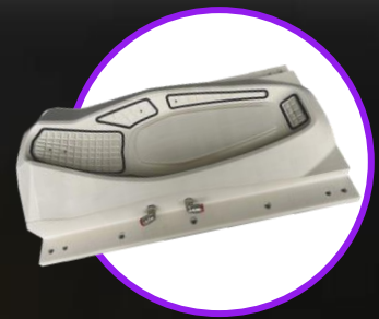
A composite tool produced by Novation Tech using a Massivit printer and Sika materials
