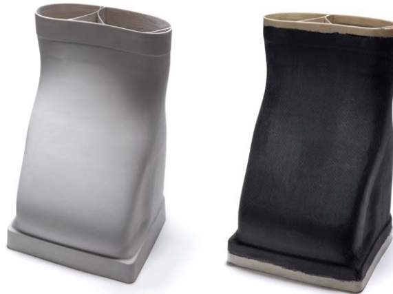
Figure 1. Full-scale mandrel (left) and resulting composite skin (right) 3D-printed with Massivit's water breakable polymer
