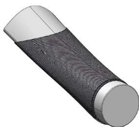
Figure 6. Mandrel wrapped with carbon fiber sheet
